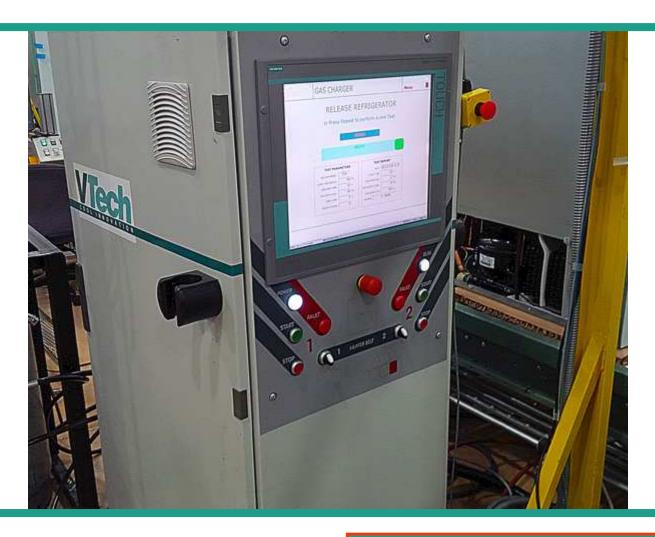
The VTech MRC Automatic Evacuation and Refrigerant Charging System is designed for HFC & HCFC refrigerants (e.g. R134a, R404a, R407c or R410a) in a production environment. The system performs an automatic vacuum cycle and a vacuum decay leak test, prior to refrigerant charging.
